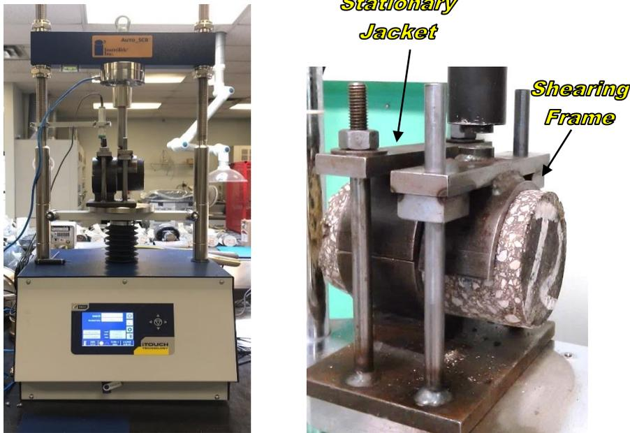
Figure 2-7 InstronTek© Testing Frame (Right) and Interlayer Shear Strength (ISS) Apparatus (Left)
