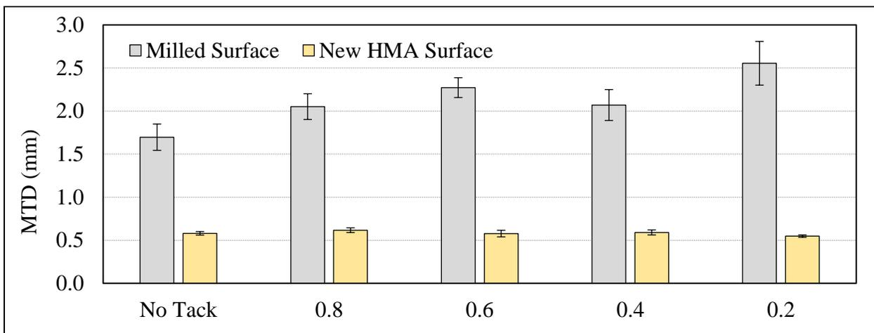
**Figure 3-3 Mean Texture Depth (MTD) Measure Using Sand Patch Test**
