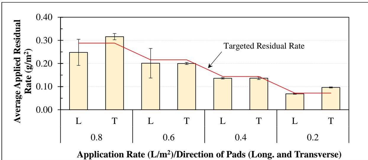
**Figure 3-2 Results of ASTM D 2995 Field Verification of Application Rates**
